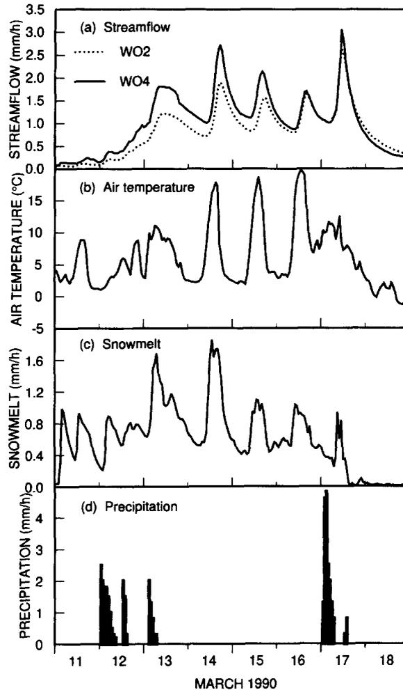
Fig. 5. Hydrologic data for March 1990 snowmelt: (a) discharge of streams WO2 and WO4; (b) air temperature from a site on the Woods Lake outlet stream; (c) rate of snowmelt from the snow lysimeter in catchment WO2 (the snowpack was gone from the lysimeter by noon on March 16; thus the lysimeter served as a throughfall collector thereafter); (d) hourly precipitation.
