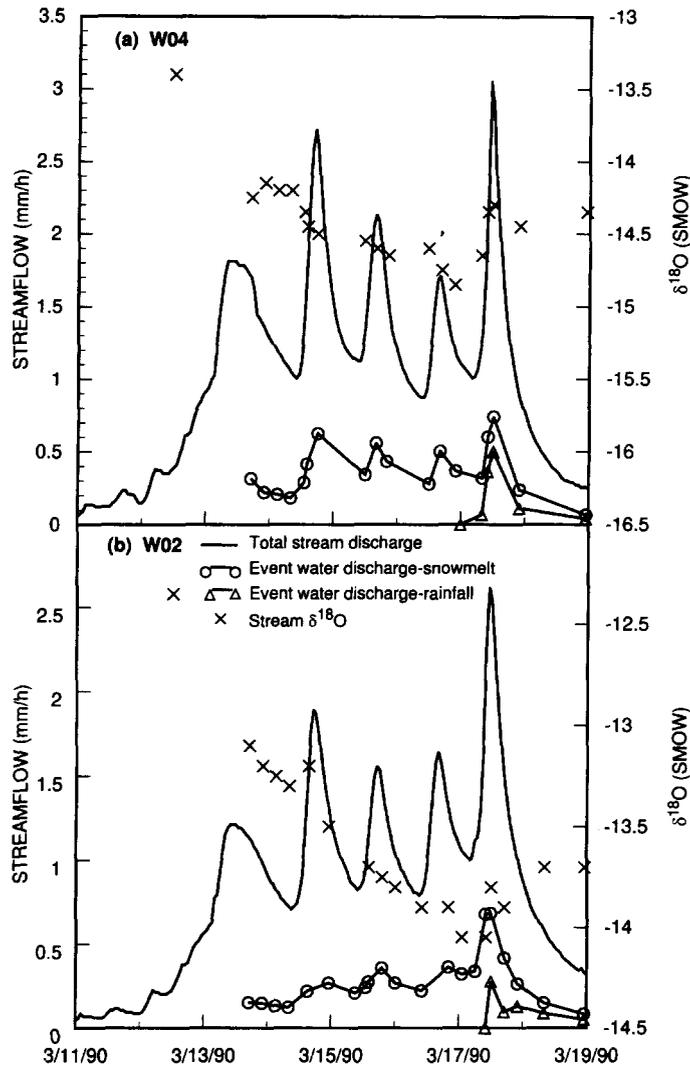
Fig. 6. Total stream discharge, event-water discharge, event-water discharge from rainfall on March 17, and  $\delta^{18}\text{O}$  of stream water during the snowmelt of March 1990: (a) stream W04; (b) stream W02.
