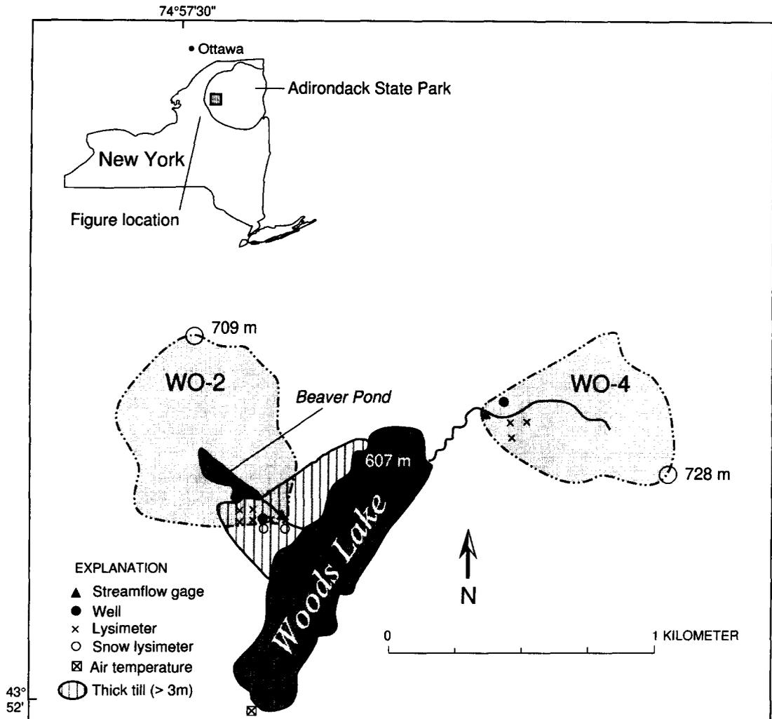
Fig. 1. Map of Woods Lake with the gaged areas of catchments WO2 and WO4 shown. Locations of the wells, soil-water lysimeters, snow lysimeters, and air temperature probe are also shown on the map.
