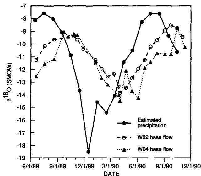
Fig. 4.  $\delta^{18}\text{O}$  data for base flow samples collected from WO2 and WO4, and estimated  $\delta^{18}\text{O}$  of composited monthly precipitation.
