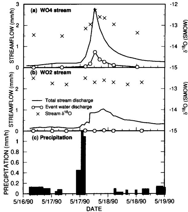
Fig. 7. Total stream discharge, event-water discharge, and  $\delta^{18}\text{O}$  of stream water during the rain event of May 1990: (a) stream WO4; (b) stream WO2; (c) hourly precipitation.
